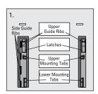
Identify attachment components in housing.
