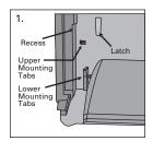
1. Identify attachment components in housing.
